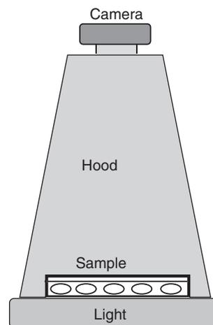
**Figure 3** Setup for digital photography of sample plate.
