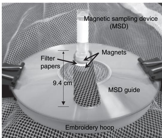
**Figure 2** Design and use of magnetic sampling device to collect insecticide residue on net surface.
